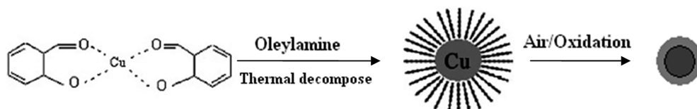
Figure 34. Schematic diagram for Cu/Cu 2 O core/shell nanoparticle synthesis using the thermal decomposition of a metal organic complex. Reaction scheme adapted from ref 569.
